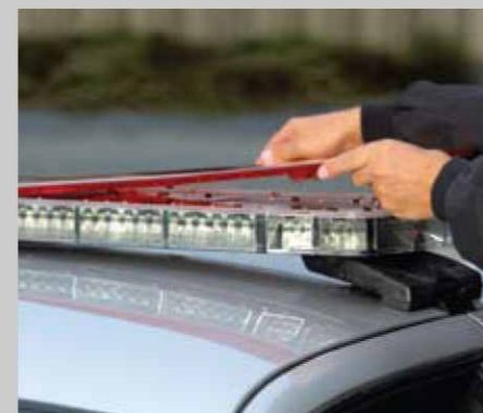
1 Remove the top dome with only four screws
