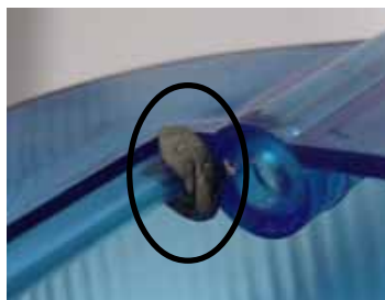
Fig 2. Wrap the sealant around the lens guide in the part to be screwed.
