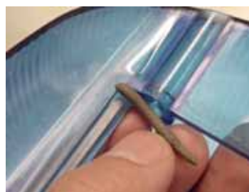
Fig 1. Take a portion of sealant Ref. 9040150 and form a tubular shape.
